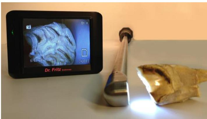
*Pic1: A digital LED endoscope for equine dentistry with wireless data transfer to a hand held monitor. Without the need for an external light source or cables, this battery powered instrument is marvelous for field practice. (Dr. Fritz endoscopy Germany).*
